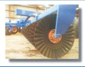
Uses existing proven features. Up To 26" discs to still provide effective cut out on 9" spacings. Choice of 3 gang angles to allow full cut out in shallow working. The Sandgroper is still a true tandem offset sics plough.
