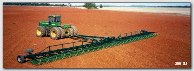
Induction hardened pins, precision machining in the universal joint, extra heavy duty frame construction and 2.5T axles have been incorporated into the design for harsh Australian field conditions.
