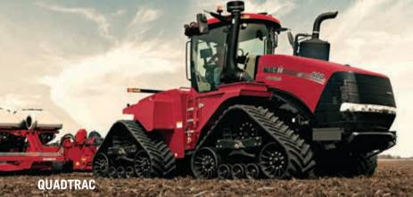
More than 20 years of industry-leading track technology can be found in every AFS Connect Steiger Quadtrac® tractor, which features four individually driven, positive-drive oscillating tracks.
