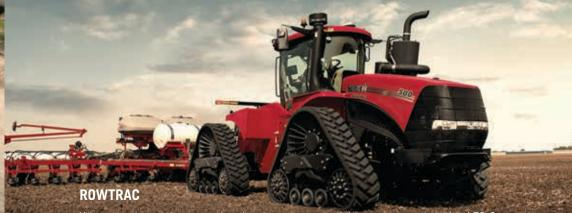
When traction and agronomic advantage are essential to your operation, the AFS Connect Steiger® Rowtrac<sup>™</sup> tractors are the right choice. These tractors offer a range of row crop track widths and axle configurations to meet your needs: 20-, 22-, 30- or 40-inch (508, 558.8, 762 or 1016 mm) rows.
