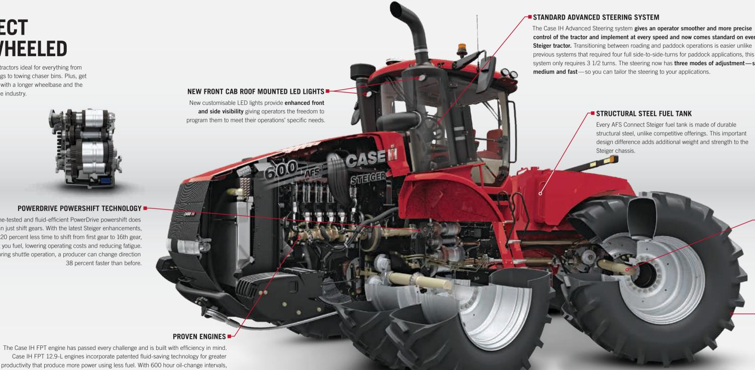
control of the tractor and implement at every speed and now comes standard on every Steiger tractor. Transitioning between roading and paddock operations is easier unlike previous systems that required four full side-to-side-turns for paddock applications, this system only requires 3 1/2 turns. The steering now has three modes of adjustment—slow, **medium and fast**—so you can tailor the steering to your applications.
