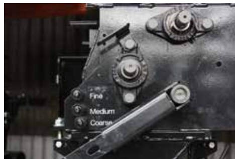
Metering Gate helps control product flow.
