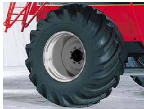
High flotation tyres reduce rolling resistance and soil compaction.
