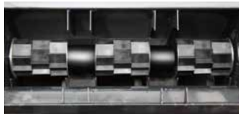
Robust fluted rollers meter fine, medium and coarse seeds and most fertilisers.
