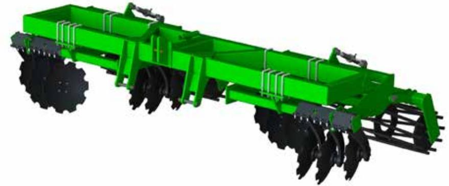
The TrackAttack<sup>®</sup> by K-Line Ag is designed to level out wheel tracks, ruts and uneven terrain. The front row of discs cut through the ground, loosening and moving the soil onto the tram-line, then the crumbler roller follows behind breaking down the soil and cloddy dirt. This leaves the tram-line with a flat and even weed free surface, making it easier and smoother for equipment to pass.
